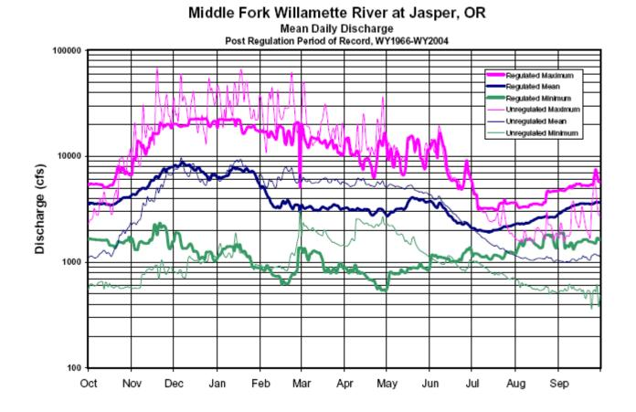
Figure 3. Mean daily discharges (maxima, minima and averages) at the Jasper gage, Middle Fork Willamette River for period of postdam completion (1966-2004). Regulated flows are those observed at the gage; unregulated flows are derived from USACE models. Figure prepared by Chris Nygaard, USACE, Portland, OR.
